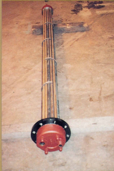
Intercooler, 5" x 7' long, completed and ready for delivery.
