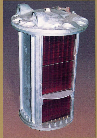
Intercooler bundle with Admiralty tubes, Copper fins and Carbon Steel tubesheets. Cast Iron side panels were reused. Tubesheets and cores are kept in stock at PES for this particular type of cooler.
