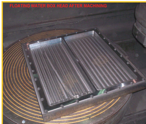
Head for a hydrogen cooler after machining
