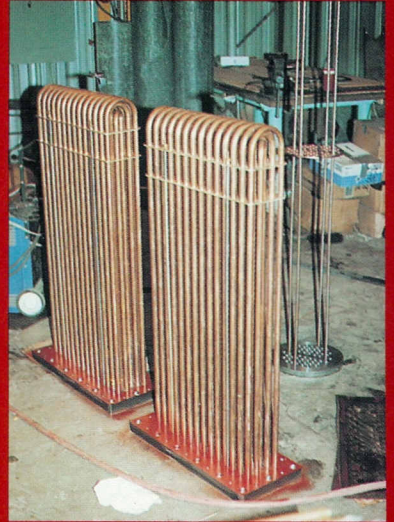
Oil cooler, U-tube design. This design is used in power plants.
