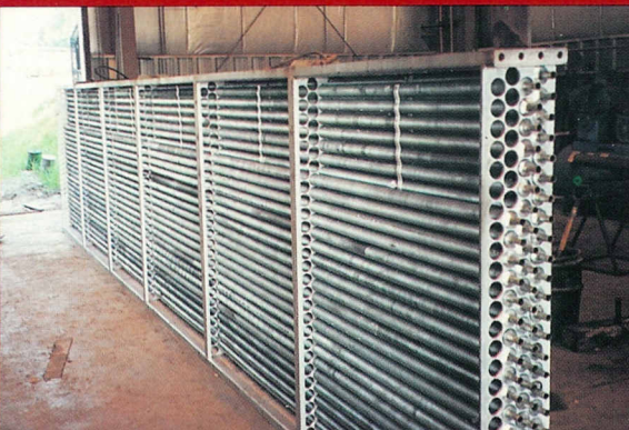
Fin-fan coils of various types and sizes are routinely handled. This unit has 1" O.D. Admiralty tubes with L-footed tension wound Aluminum fins.
