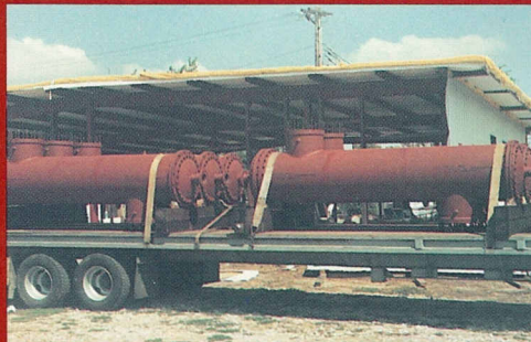
Series of five large aftercooler units. New bundles were installed after shells were reconditioned. These units were delivered to a large pharmaceutical company on PES owned and operated vehicles.
