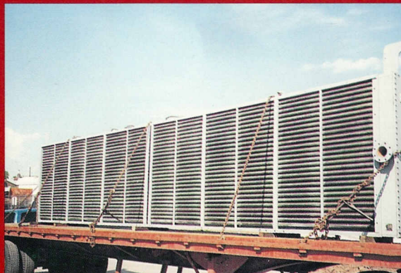
Fin-fan coil completed and ready for delivery.
