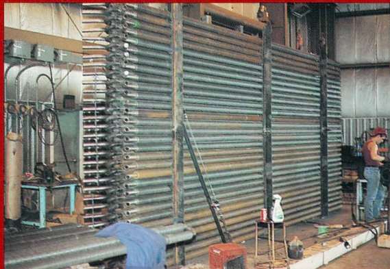
Large scrubber coil assembly for use in a power plant. Unit size is approximately 2' x 11' x 26'. Constructed of Carbon Steel with high-finned tubes.
