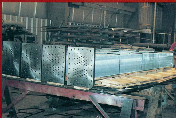
Hydrogen cooler with sheet fin design. These coolers can also be supplied with wrap-on fins in a variety of materials.
